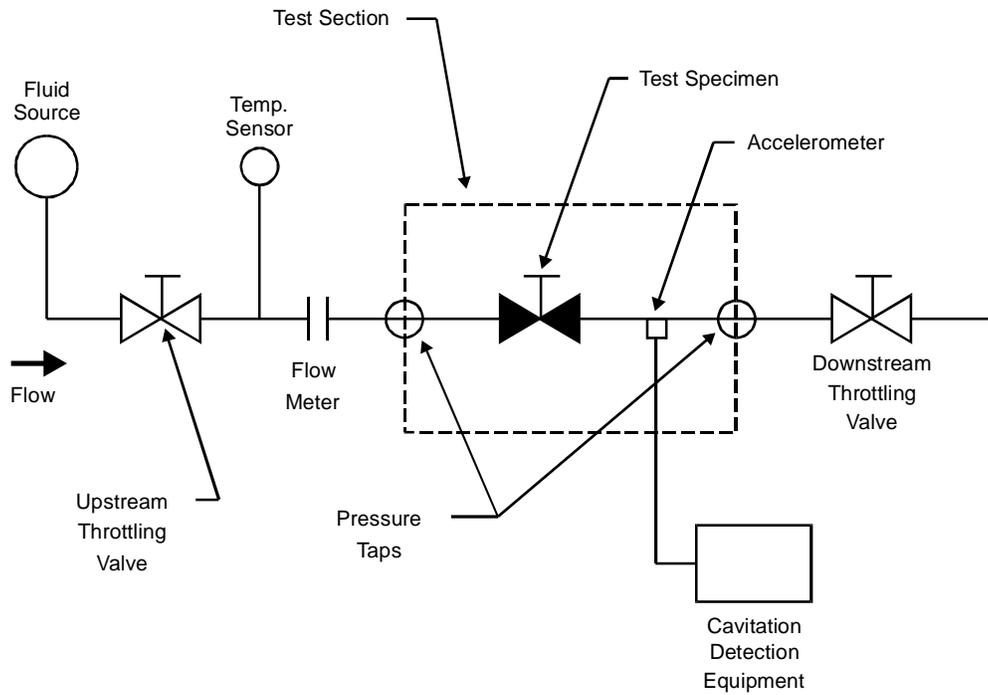
**Figure 2 — Flow test system**
