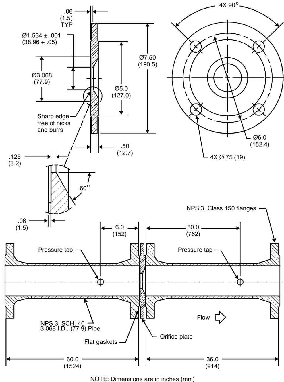
Figure 4 — Cavitation calibration test manifold
