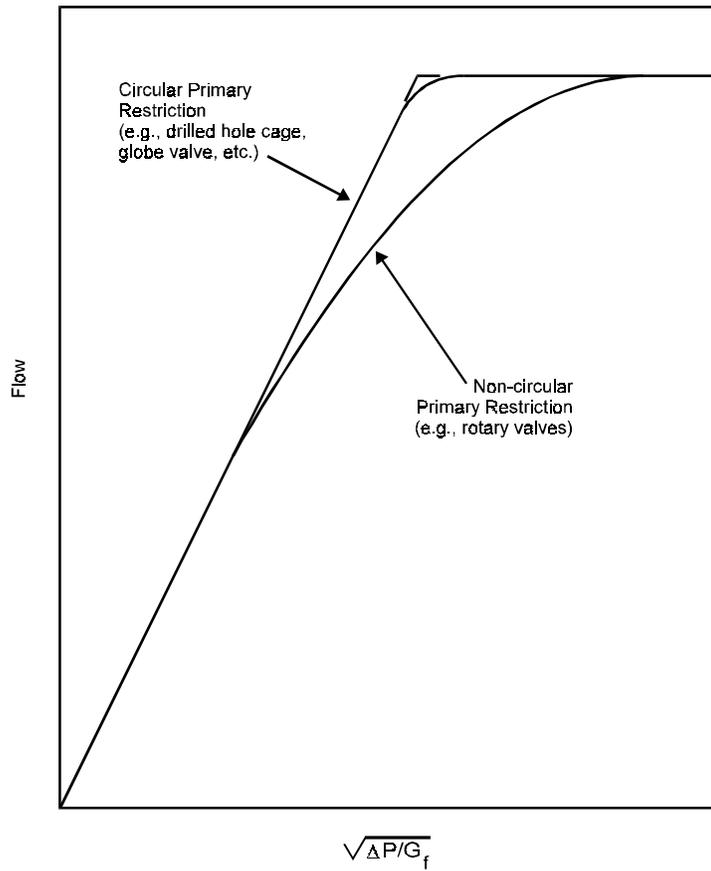
**Figure B.3 — Typical flow curve appearance**
