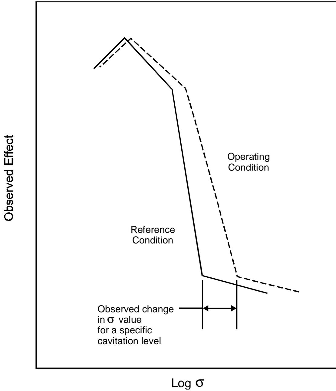
**Figure B.1 — Cavitation scale effects**
