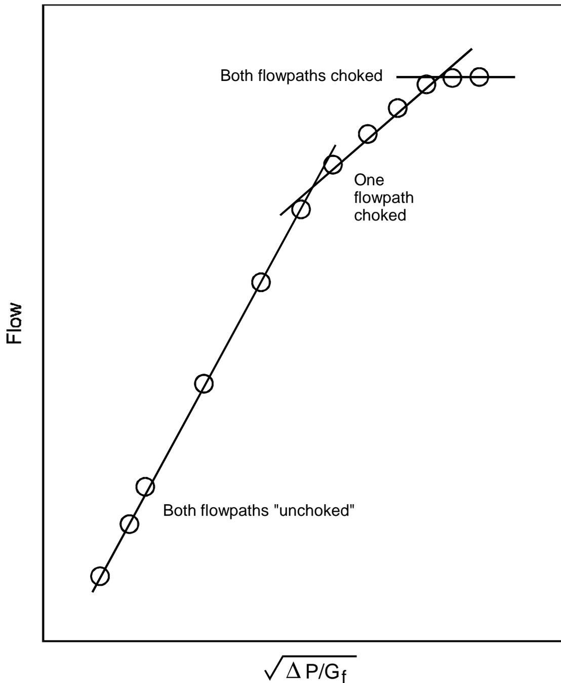
**Figure B.4 — Flow curve appearance: two flowpath butterfly valve**
